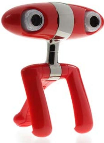
at you when the standard USB 2.0 connection is plugged into a computer. Each eye of the Minoru is a camera. The webcam performs stereoscopic anaglyphic processing to sew the two separate images into a 3D image stream at up to 30 frames per second.
